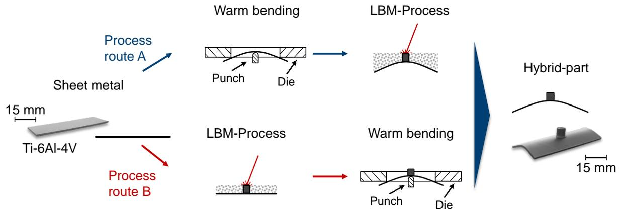
**Figure 1** : Process routes for manufacturing of hybrid parts by combining LBM and sheet metal forming
