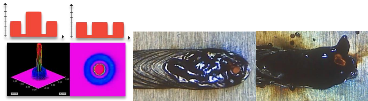
(a) Beam mode of ARM laser (b) Laser welding with ARM laser (c) Laser welding with normal laser Fig. 1. ARM laser beam mode with center and ring powers, and comparison of molten pool and keyhole behavior during welding of A6XXX aluminum alloy with ARM laser and normal laser.
