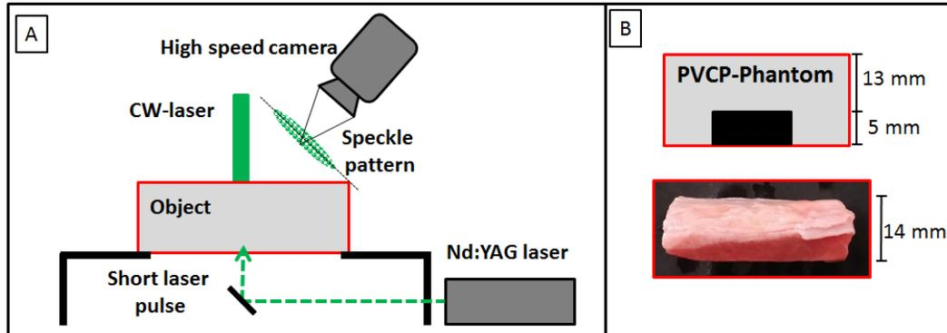
Figure 1. A: The object is excited with a short laser pulse and the speckle pattern is acquired with a high-speed camera. B: The sample geometries are shown
